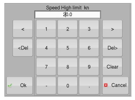
This example show the "Speed High limit" that is set to 20.0 kn.
