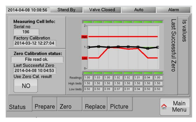
The graph indicates eight different values measured in the Measuring Cell. Values from the left are: #1 internal reference, #2-6 photo diodes, #7 water detector, #8 temperature.
